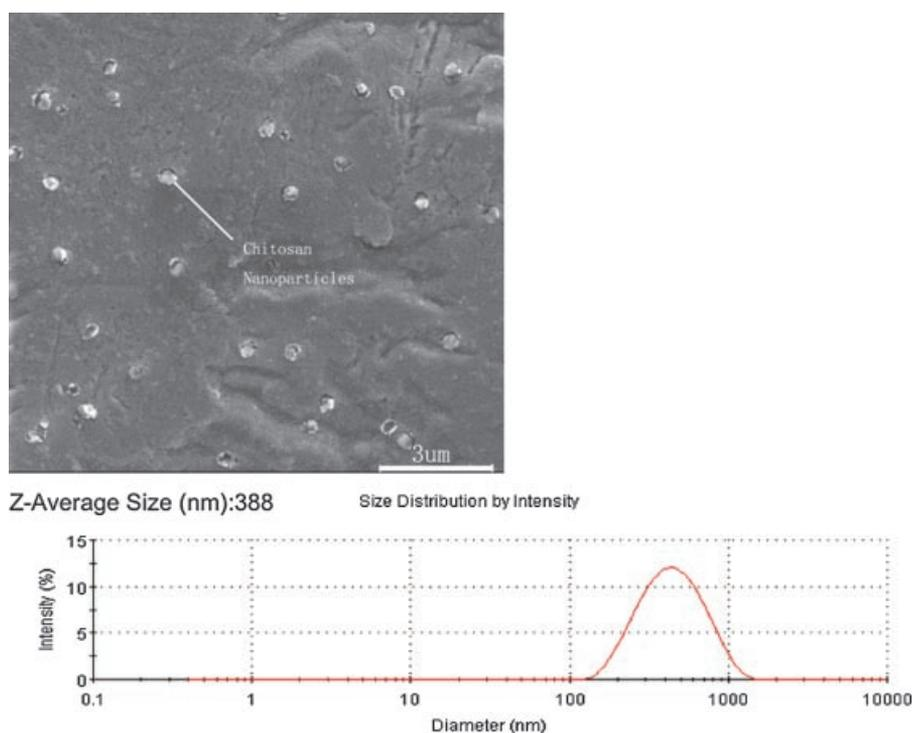
**Figure 1.** a: Typical SEM image of Chitosan nanoparticles containing Rhodamine B. b: Size distribution of Chitosan nanoparticles containing Rhodamine B; Scale bar is 3 μm.
