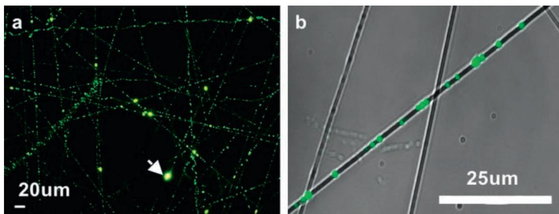
**Figure 3.** a: Fluorescent image of Chitosan nanoparticles-FITC/PCL core-sheath nanofibers. b: LSCM image of Chitosan nanoparticles-FITC/PCL core-sheath nanofibers; Chitosan nanoparticles labeled FITC shows green light.
