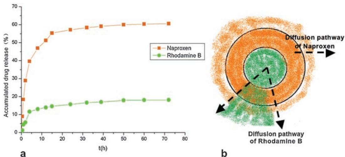
**Figure 4.** a: Release behavior of Rhodamine B and Naproxen from Chitosan nanoparticles/PCL electrospun nanofibers with core-sheath structures. b: Scheme of diffusion pathway of Rhodamine B and Naproxen from core-sheath electrospun nanofibers, Orange color—Naproxen, and Green color—Rhodamine B.
