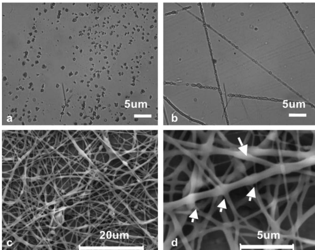
**Figure 2.** a: LM image (40 $\times$ ) of Chitosan nanoparticles encapsulating Rhodamine B. b: The LM image (40 $\times$ ) of Chitosan nanoparticles/PCL composted core–sheath electrospun fibers, Chitosan nanoparticles encapsulating Rhodamine B (Core) and PCL embedding Naproxen (Sheath). c and d: The SEM image of Chitosan nanoparticles/PCL composted core–sheath electrospun fibers.
