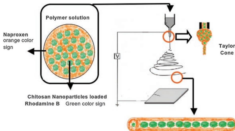
**Scheme 1.** Schematic illustration of method for preparing core–sheath nanofibers containing chitosan nanoparticles encapsulating Rhodamine B (as core). Naproxen was embedded into the sheath. Multiple agent loading in different site of this core–sheath nanofiber can provide independent control over the release of each agent.
