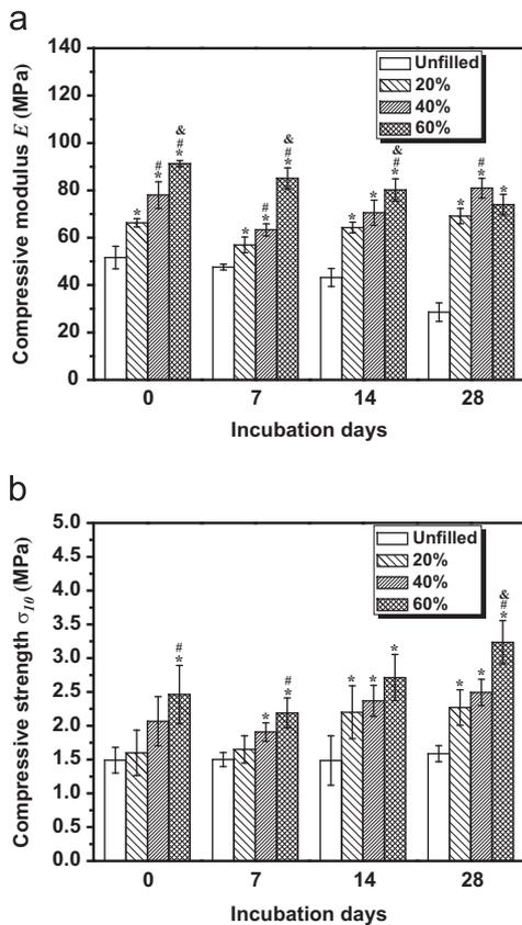
Fig. 7 – (a) Changes in compressive moduli ( $E$ ) and (b) strengths ( $\sigma_{10}$ ) of the PDLLA scaffolds with different amounts of nano-HAp after incubation in SBF for different time. Results are mean  $\pm$  SD. \*, #, & indicate statistically significant difference as compared with unfilled PDLLA, PDLLA with 20 wt% and 40 wt% of nano-HAp, respectively ( $n=5$ ,  $p < 0.05$ ).
