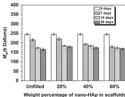
**Fig. 5** – Weight average molecular weight ( $M_w$ ) changes of PDLLA scaffolds with 0, 20, 40, 60 wt% of nano-HAP after incubation in SBF for different time periods. Results are mean  $\pm$  SD. \*, #, and & indicate statistically significant difference as compared with 0 day, 7 days, and 14 days, respectively ( $n=3$ ,  $p<0.05$ ).
