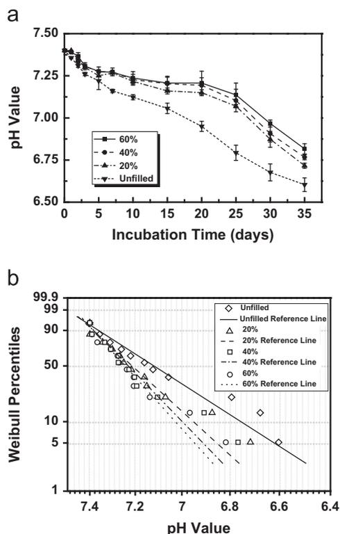
Fig. 9 – The pH changes of PBS after immersion of PDLLA scaffolds with 0, 20, 40, 60 wt% of nano-HAp, (a) pH versus incubation time and (b) the Weibull probability plot of pH value data.
