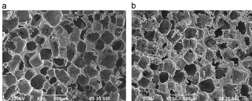
Fig. 1 – SEM micrographs of porous scaffolds before incubation in SBF: (a) unfilled PDLLA and (b) PDLLA filled with 60 wt% of nano-HAp.
