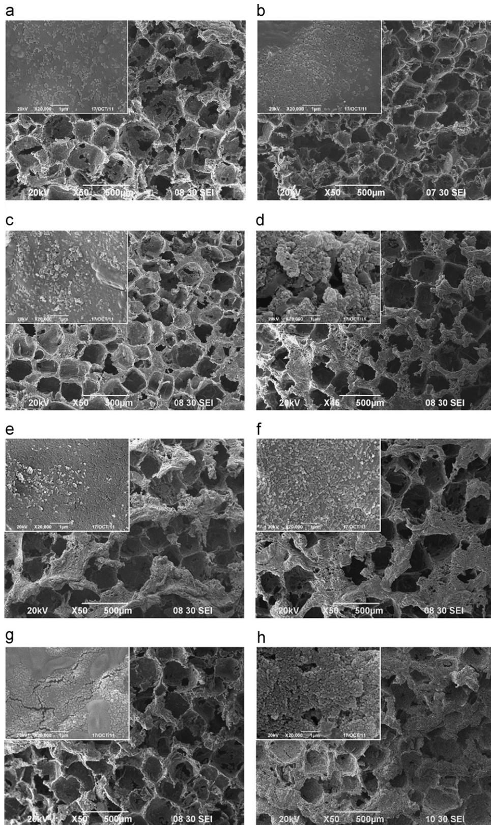
**Fig. 2 – SEM micrographs of porous scaffolds after incubation in SBF for (a–d) 7 days and (e–h) 28 days at low and high magnification: (a, e) unfilled PDLLA, PDLLA filled with (b, f) 20 wt%, (c, g) 40 wt%, and (d, h) 60 wt% of nano-HAP.**
