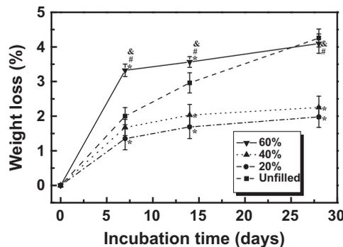
**Fig. 6** – Weight losses of the PDLLA scaffolds filled with different amounts of nano-HAP (0, 20, 40, and 60 wt%) after incubation in SBF for different time periods. Results are mean  $\pm$  SD. \*, # and & indicate statistically significant difference as compared with unfilled scaffold, 20 wt% and 40 wt% nano-HAP filled PDLLA scaffolds, respectively ( $n=3$ ,  $p<0.05$ ).
