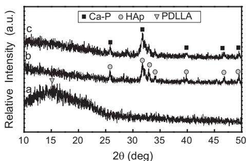
**Fig. 4** – TF-XRD graphs of (a) unfilled PDLLA scaffold before immersion in SBF; (b) PDLLA/60 wt% nano-HAP scaffold before immersion in SBF; and (c) PDLLA/60 wt% nano-HAP scaffold after immersion in SBF for 28 days.
