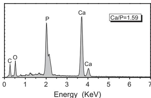
**Fig. 3** – EDX spectrum for confirming the presence of apatite formation on the surface of the PDLLA/60 wt% nano-HAP composite scaffold after incubation in SBF at 37 °C for 28 days.
