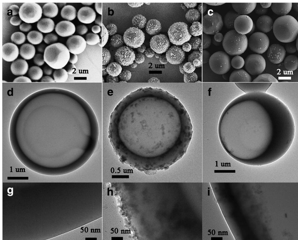
**Fig. 1.** SEM images of (a) blank microbubbles, (b) SPIO-coated microbubbles, (c) SPIO-embedded microbubbles, TEM images of (d) blank microbubble, (e) SPIO-coated microbubble, (f) SPIO-embedded microbubble, (g–i) are partially enlarged images of (d–f).
