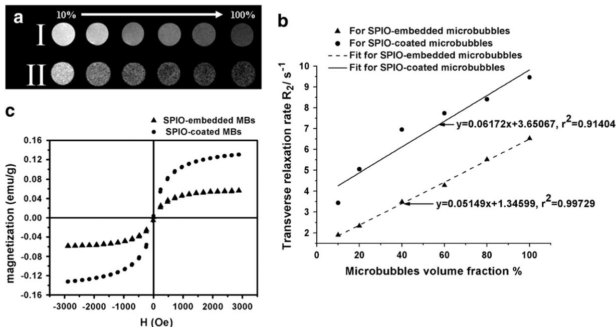
Fig. 3. (a) MR images of SPIO-embedded microbubbles (I), SPIO-coated microbubbles (II); relationship between  $R_2$  and volume fraction of two types of microbubbles (b), and (c) hysteresis loops of (I) and (II).
