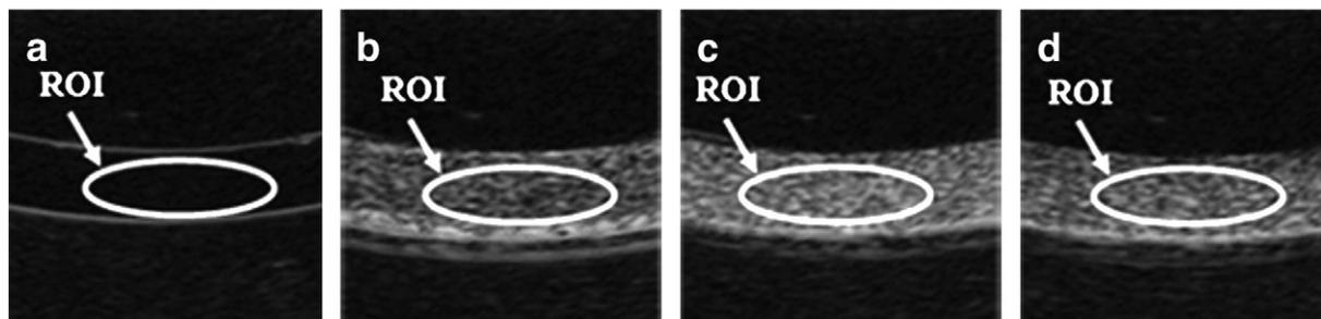
Fig. 2. B-mode ultrasound images of (a) distilled water, (b) blank microbubbles, (c) SPIO-coated microbubbles and (d) SPIO-embedded microbubbles.
